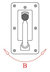
If There Is Any Movement In The Direction Of Arrows "A" Or "B" Use The Following Procedure To Re-Tighten.
